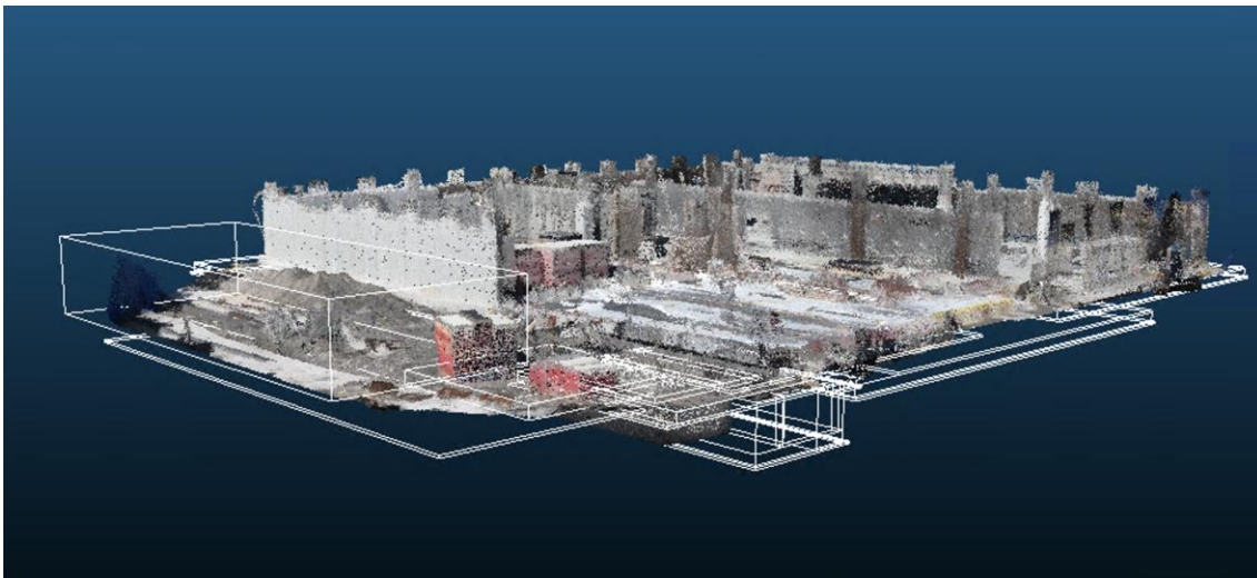
Figure 47. Mapping between the IFC elements and construction point cloud data – Polish pilot
